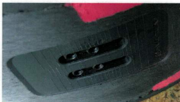
FIGURA 5 – DESNIVEL DE 1 MM EN FIVE TEN KESTREL LACE
